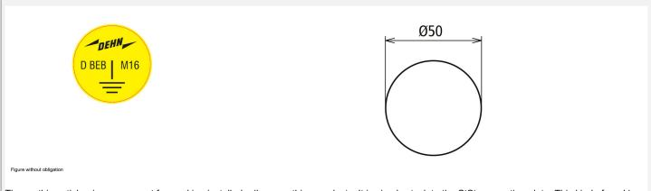
The earthing sticker is a spare part for marking installed railway earthing products. It is simply stuck to the StSt connection plate. This kind of marking can be used for earthing bridges D BEB 1 to 8 as well as for the D BEB 11 version for earthing large pipes if the sticker applied in the factory has fallen off or is damaged.
