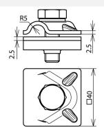
Multipurpose connecting clamp with spring washer for universal use as cross, T and parallel clamp; two-piece design. Tested for lightning current carrying capability up to 200 kA ( $10/350 \mu s$ ).
