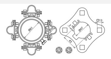
Fixing kit for installation of the HVI long Conductor on HVI supporting tubes, consisting of a connection plate (for four conductors, incl. two serrated lock nuts) and a fixing ring with four slotted conductor holders (Ø20 mm) for the sealing end (incl. two cable ties).
