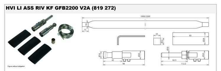
Connection kit for sealing the HVI light Conductor at both ends, for implementing the adjustment range of the conductor in the supporting tube (head piece) and connection element for other parts of the external lightning protection system or earth-termination system (incl. EB connection cable, constant force spring and three heat-shrinkable sleeves).
